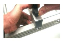
Rotate the end of the hook under the lip of the frame rail and tighten the knob while holding the end of the hook in place. Repeat this procedure of the other hook on the rack. Install the other rack to the frame about 41/1.2m from the other rack
