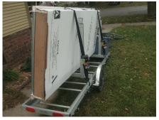
Place your cargo (plywood, sheetrock, etc.) on the angle stops and lean it again the padded surface of the pivot blocks. Tie down your load using ratchet straps (preferred) or shock cords. You may want to insert some pieces of cardboard or similar soft material between your cargo and the stops and straps to prevent the edges from damage.
