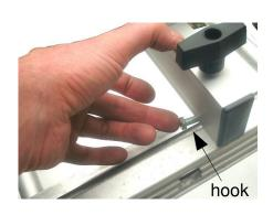
Place one of the racks across the trailer frame with the end of the hook perpendicular to the base and parallel to the trailer frame side rails.
